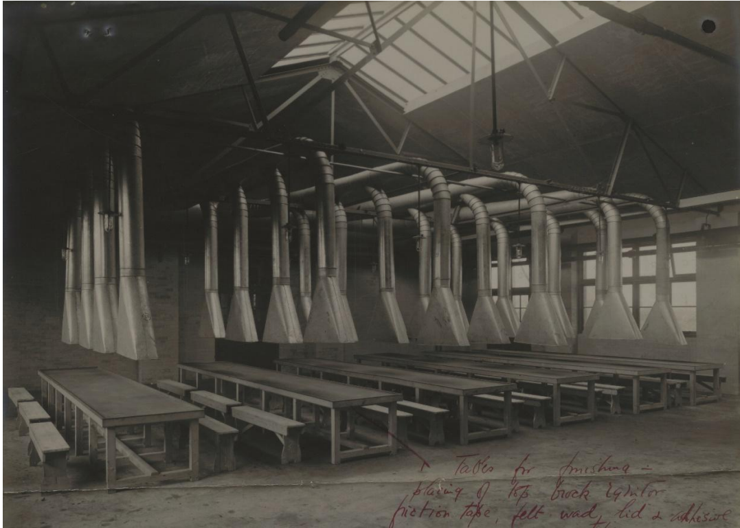
Fig 8. View of the finishes shed. Tables for finishing – placing the top brock ignitor, friction tape, felt wadding, lid and adhesive. TNA WO 142/116 CWO 114
